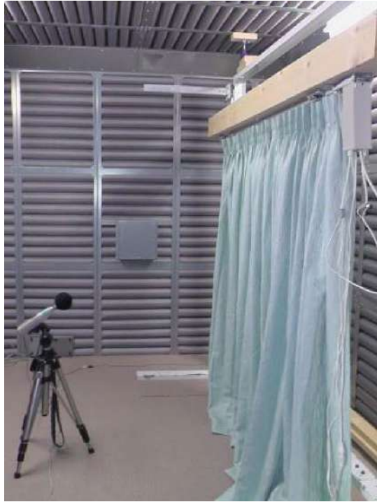
Acoustic Evaluation During 10K Test for TOSO CM2000 + Powerful Motorized Curtain Rail
