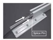
Inset the other Track into the OT Splice. (If insertion is difficult, cover the Pulley with a cloth and tap with a wooden hammer or similar tool.)
