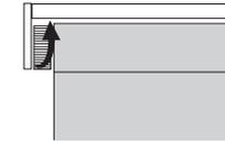
Stop the screen at the halfway up (or down) position and turn the dial as if rolling it away from you.
