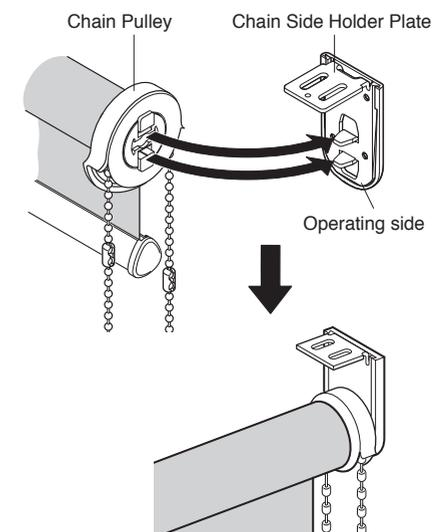
3) Put Pipe End on End Side Holder (on the opposite side), as Chain Pulley not to fall out from Chain Side Holder Plate.
