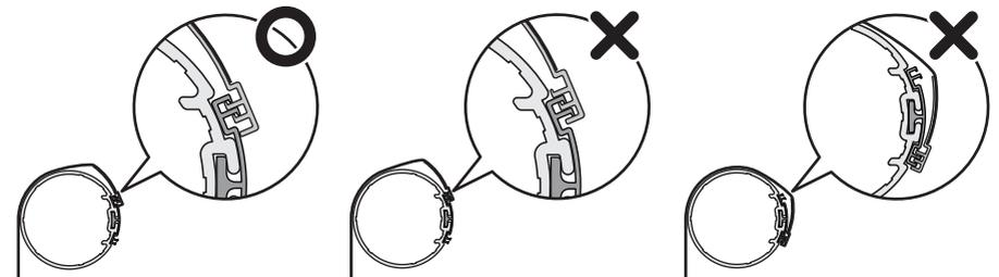
(5) Pull the chain till roll the screen up to the bottom. Mount the screen assembly onto the brackets as in Step (3) on Page 8.
