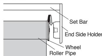
(5) Mount the screen assembly onto the brackets following Step (3) on Page 8.
