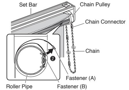
(3) Turn Set Bar so that the operating chain is positioned on the left-hand side. Pull the chain again until Chain Connector touches Chain Cover.
