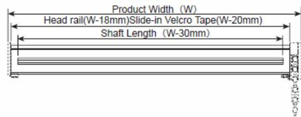
\* When cutting the head rail, be sure to remove the slide-in Velcro tape in advance from the rail. Also cut the slide-in Velcro tape separately using a utility knife or scissors.
